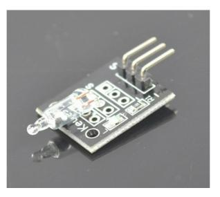
Mercury switch module and a digital interface, built-in 13 LED build a simple circuit to produce tilt warning lamp
