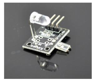
This project uses bright infrared (IR) LED and a phototransistor to detect the pulse of the finger, a red LED flashes with each pulse.
