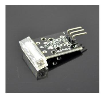
13 knock sensor module and a digital interface, built-in LED build a simple circuit to produce percussion flasher.
